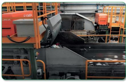
The cutting-edge, modern, energy efficient installed equipments, include different bottles and flakes detector sets as well as laser sorting units.
